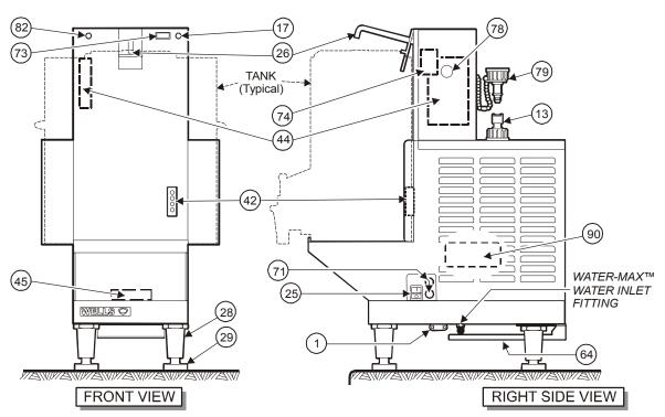
Fig. 1 Features & Operating Controls - Water Max™ Dispenser
